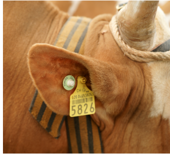
(a) RFID tag used for animal identification [credits: Sandstein/Creative Commons].
