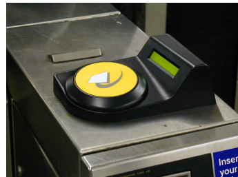
(e) An RFID reader for Oyster cards, used in public transportation in London [credits: Tom Page/Creative Commons].
