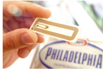
(b) RFID tag used for product tracking [public domain].
