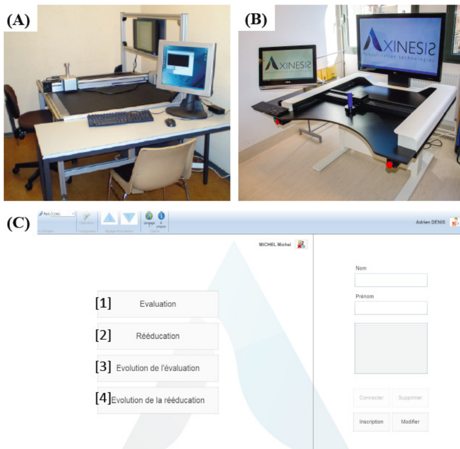
Figure 4: Illustrations of the (A) previous and (B) actual versions of the REAplan robot. (C) Presentation of the main menu displayed on the therapist's interface, which enables the clinician to (right column) connect the patient and (left column) choose a therapeutic action ([1] assessment, [2] rehabilitation, [3] assessment evolution, and [4] rehabilitation evolution).
