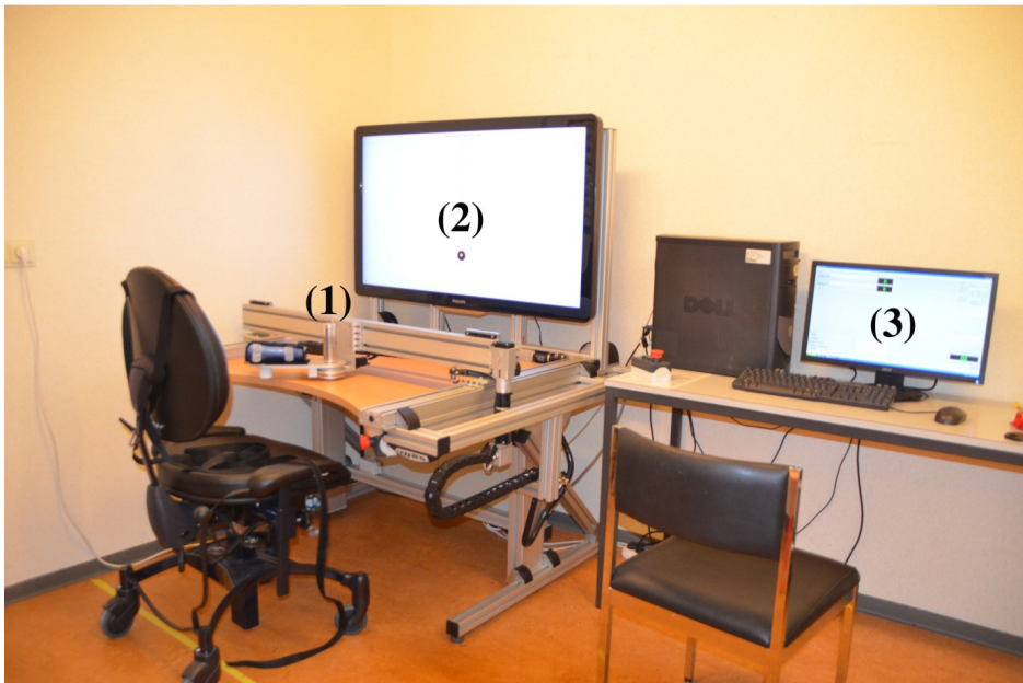
Figure 1: View of the REAplan. 1: planar end-effector robot; 2: visual interface for the subject; 3: physiotherapist's interface.
