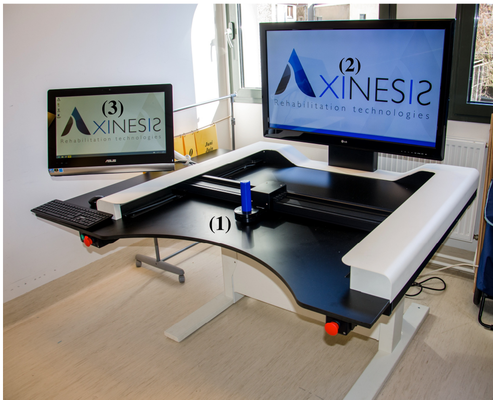
Figure 2: View of the REAplan. 1: planar end-effector robot; 2: visual interface for the subject; 3: physiotherapist's interface.
