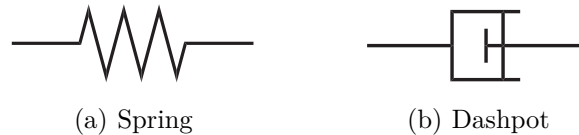
Figure 3.10 – Diagrammatic representations of ideal rheological behaviours: (a) the Hookean spring (a) and the Newtonian dashpot (b).
