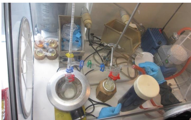
Figure 3.1 – The photo of the nitrogen-filled Plexiglas glove box, specially equipped for \text{Al}(\text{BH}_4)_3 synthesis.
