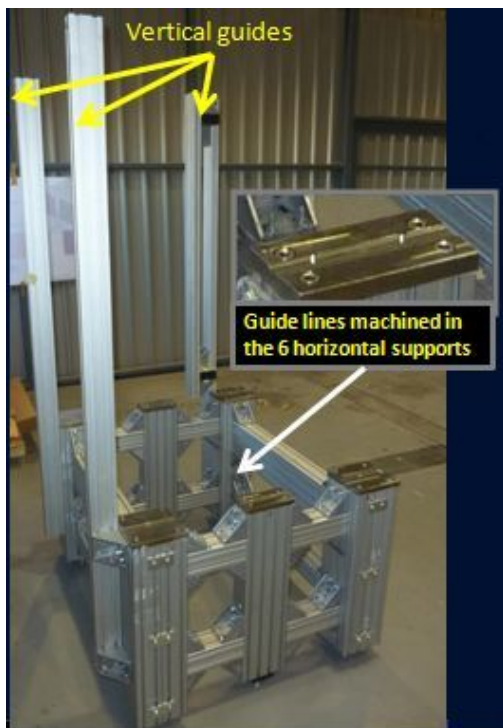
Figure 29: Left: Table for the mechanical structure assembly. It contains horizontal and vertical guide lines. Right: Detail of one corner during the assembly.
