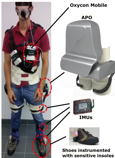
Fig. 4. Frontal view of a person wearing the experimental setup. The following components are visible: Oxycon Mobile, APO, the sensory system with inertial measurement units, and the shoes instrumented with custom pressure-sensitive insoles. For more details on the latter two, see [30].
