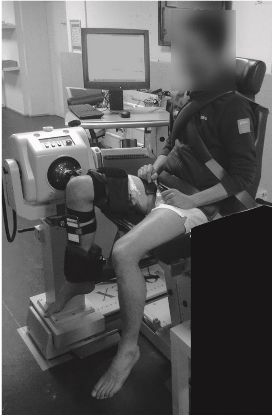
Figure 3-8 Experimental set-up using the isokinetic dynamometer and smartphone placed at the anterior medial surface of the tibia [121].
