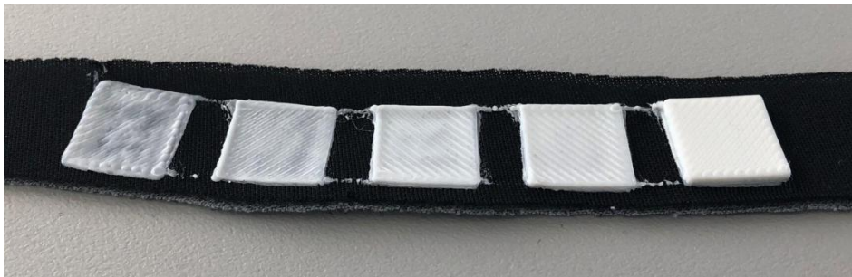
Figure 6-11 The stability changes under different ground layer thickness. From left to right, the thicker ground layer provides more stable contact interface.
