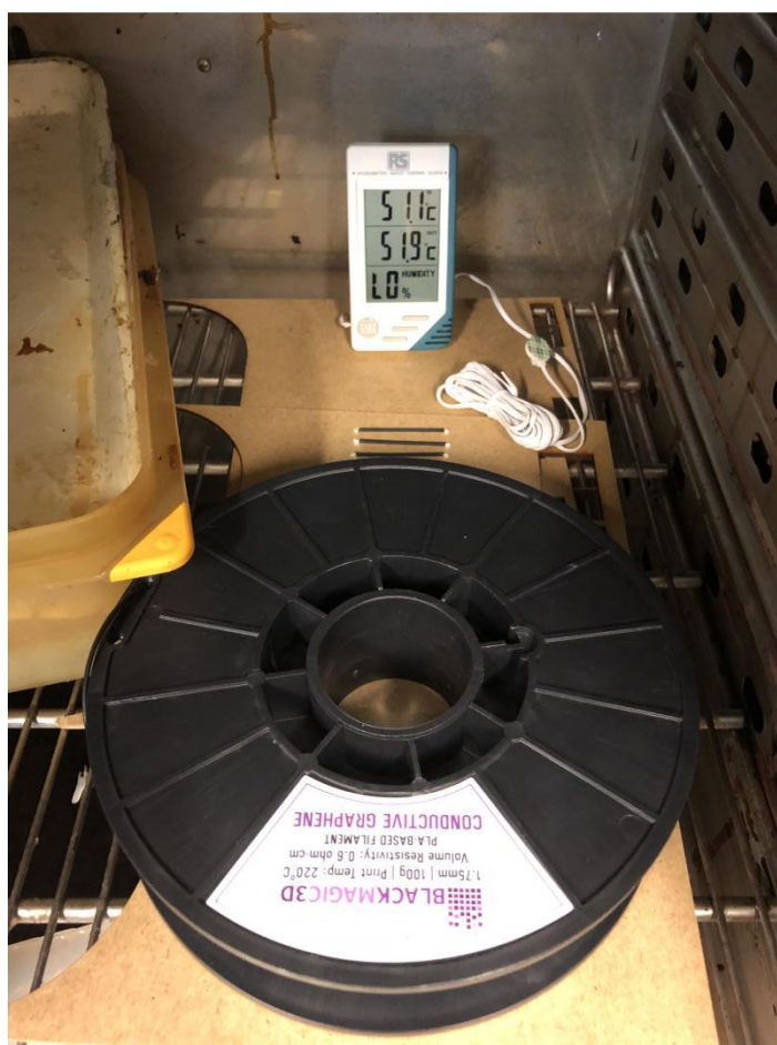
Figure 5-23 Conductive filament in the oven to remove moisture.
