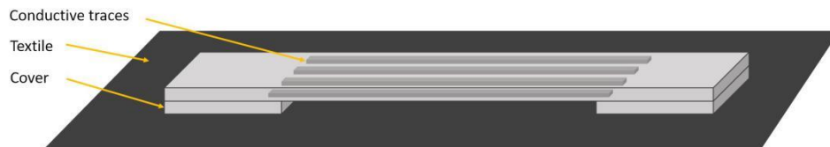
Figure 6-5 Z-axis orientation of covers contacted with the textile.
