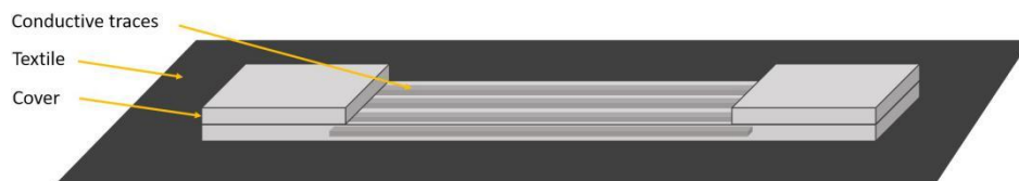
Figure 6-6 Z-axis orientation of trace board contacted with the textile.
