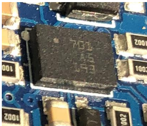
Figure 4-12 Orientation dot on BNO055.
