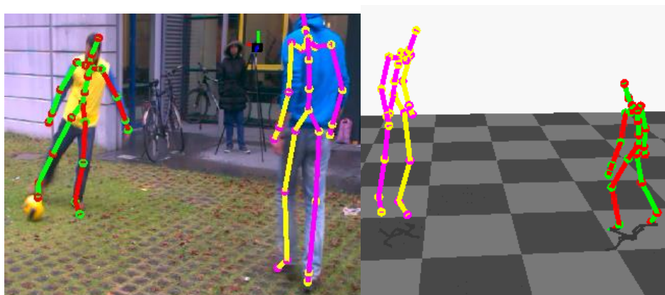
Figure 3-5 A ConvNet-based marker-less motion capture algorithm reconstructs joint angles of multiple people performing complex motions in outdoor settings, such as in this scene recorded with only three mobile phones: (left) 3D pose overlaid with one camera view, (right) 3D visualization of captured skeletons [102].
