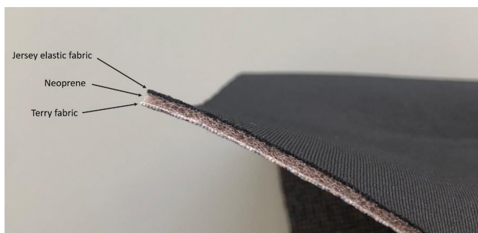
Figure 6-1 Sandwich structure of Neoprene.
