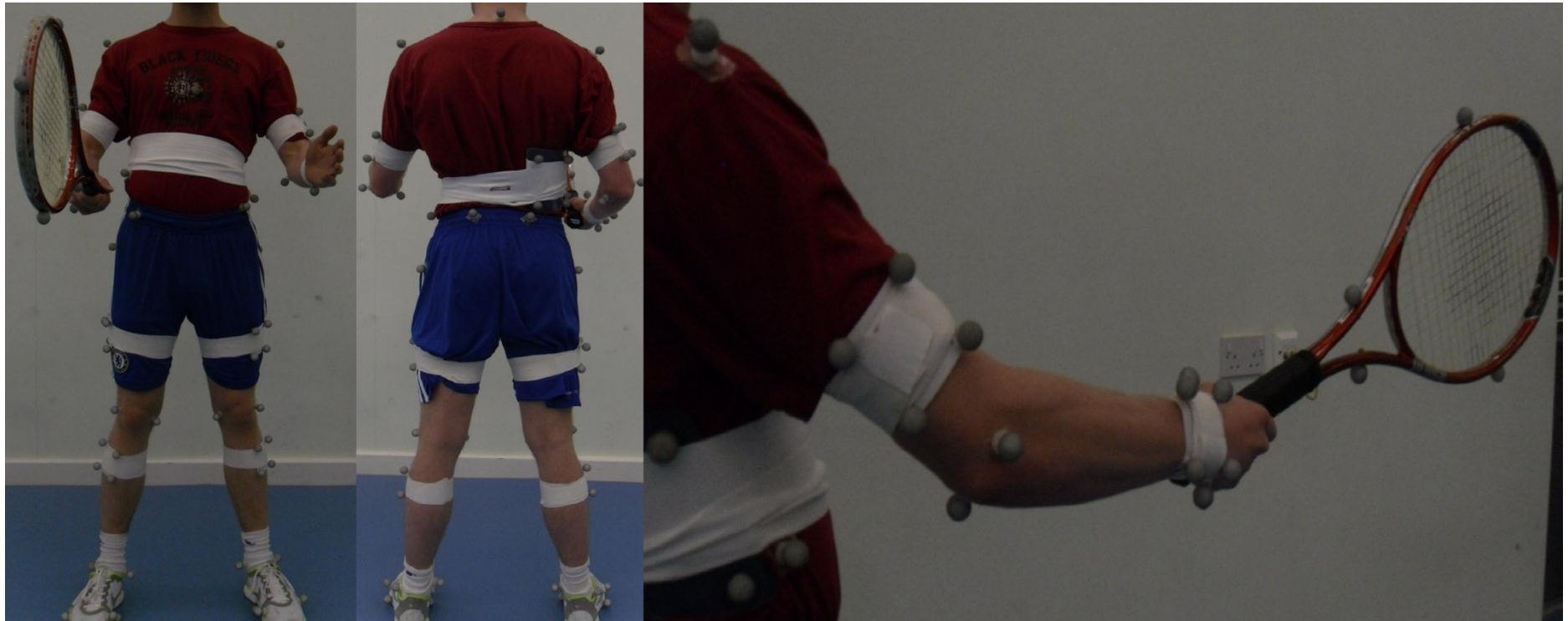
Figure 4.7 – Position of anatomical and technical markers (size 19mm diameter).
