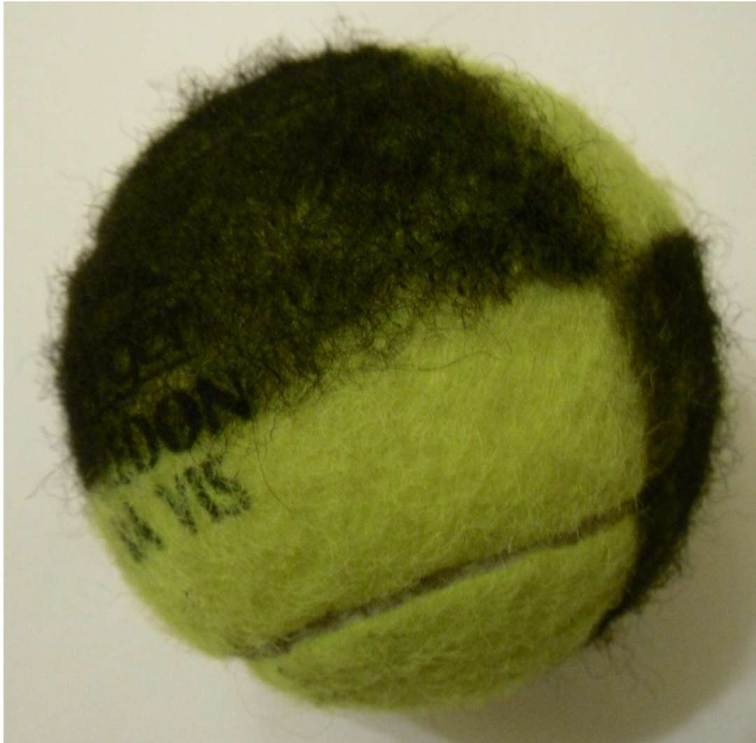
Figure 3.9 – Pattern of paint used on the ball that allowed the spin rate to be calculated most frequently
