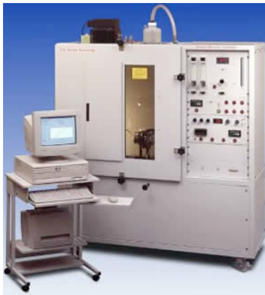
Figure 24 Example image of an FTT supplied smoke chamber. Image is taken from the FTT web catalogue
