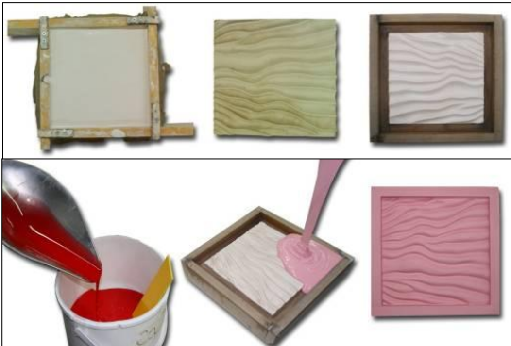
Figure 9.33: Process of mould making for the casting the tiles – creating a silicon rubber mould from a plaster cast.
