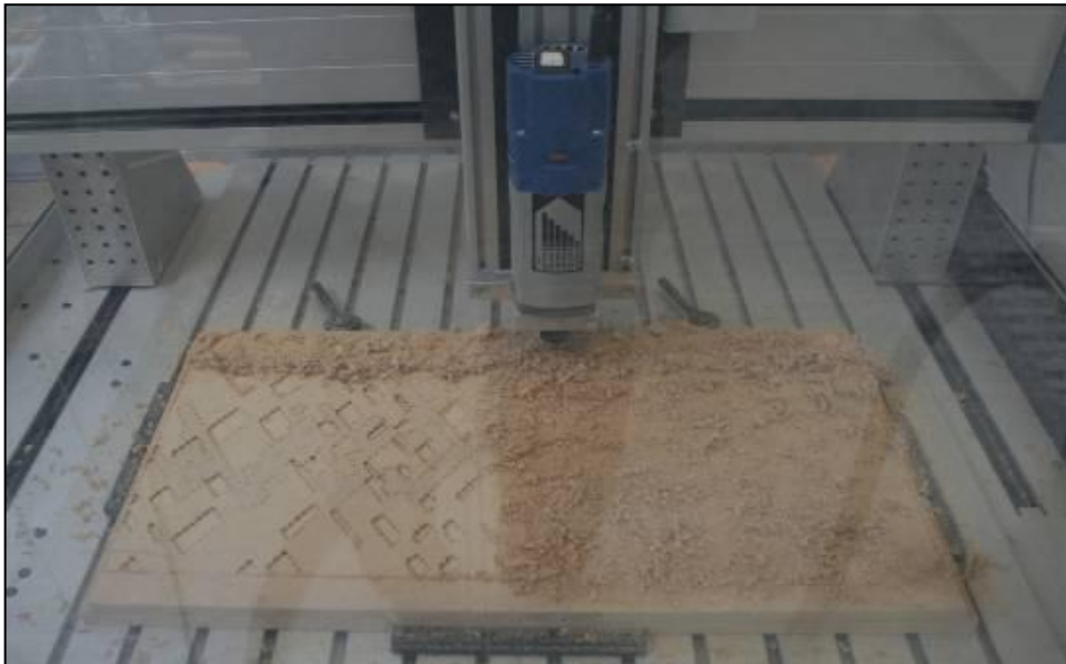
Figure 9.82: The CNC machine milling out the design in sheet MDF.
