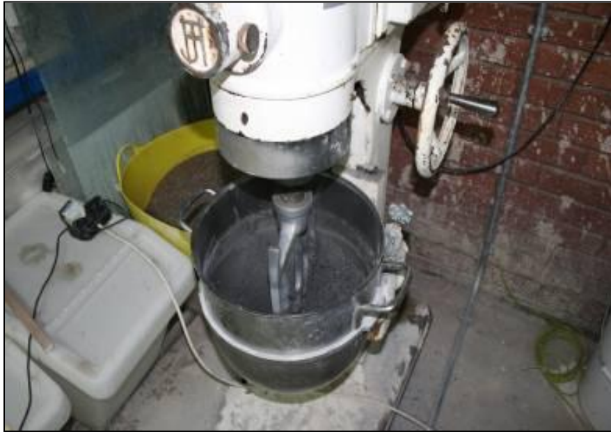
Figure 9.52: Mixing Refractory Concrete.
