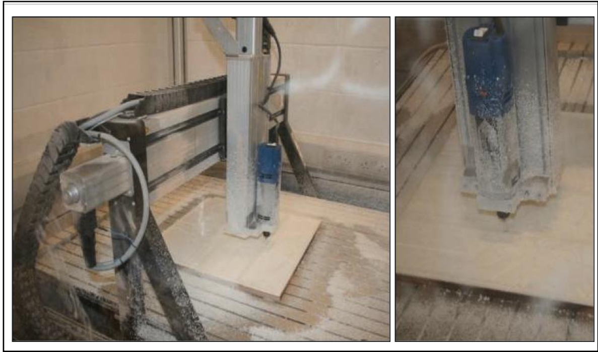
Figure 9.10: CNC Rapid Prototyping machine cutting the acrylic square.
