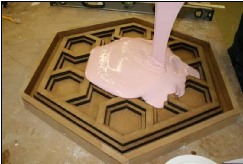
Figure 9.50: Pouring silicone rubber over MDF model.
