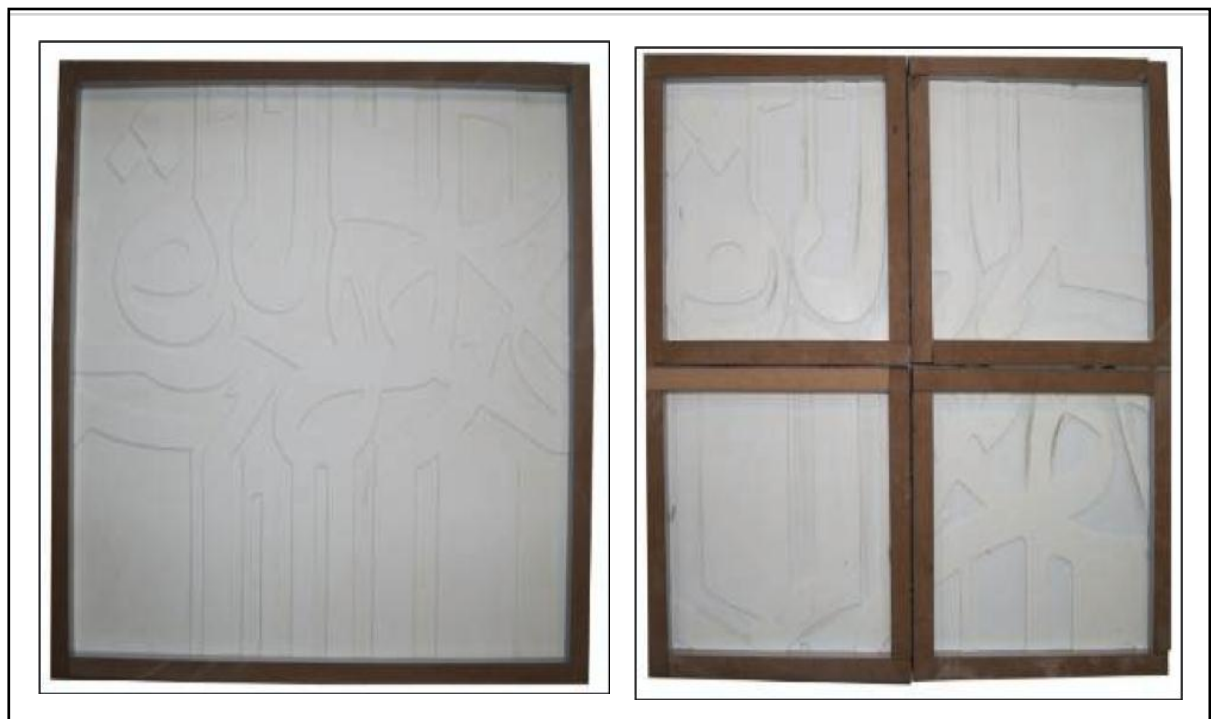
Figure 9. 11: Finished milled acrylic sheets set in wooden frames ready for casting.
