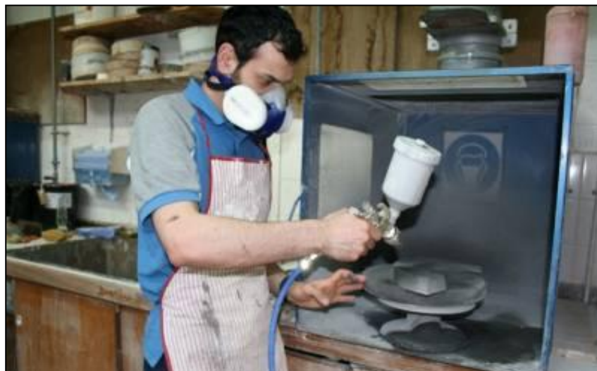
Figure 9.72: Spraying the glaze on the biscuit fired tiles.
