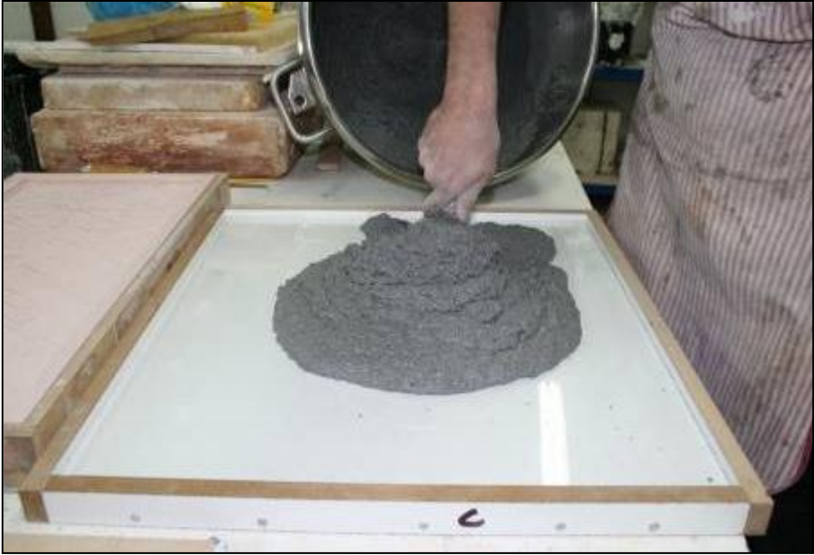
Figure 9.94: Casting refractory concrete into acrylic faced mould.
