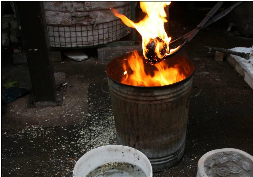
Figure 9.123: Placing Muqarnas forms in dustbin containing sawdust in order to create lustre.
