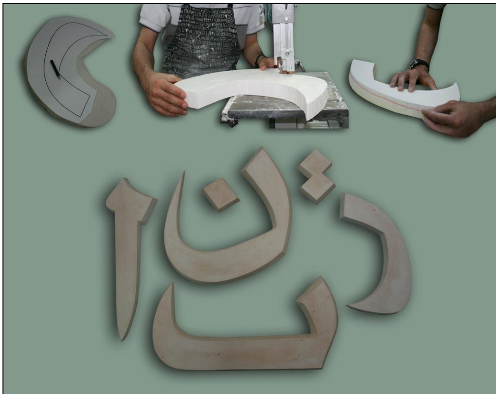
Figure 9.68: Process of creating plaster models of calligraphy letter-forms and completed set of plaster models.
