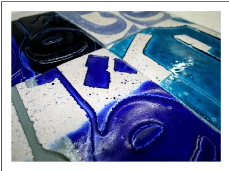
Figure 9.16: Detail of sample casts, showing ground back areas – revealing contrasting white concrete body.
