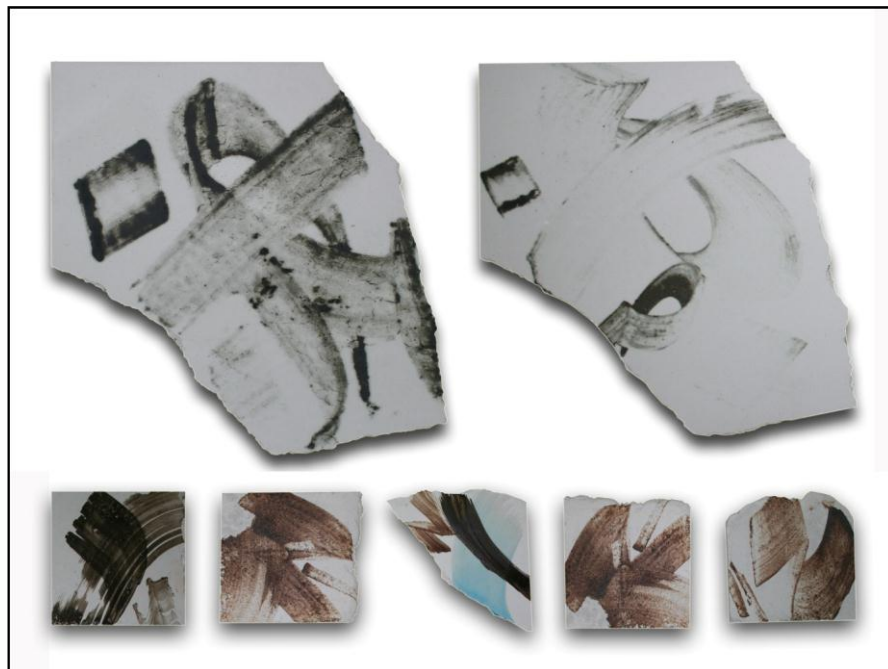
Figure 9.96: Calligraphy brushwork tests: top row fired at 1180°C, bottom row at 1080°C.
