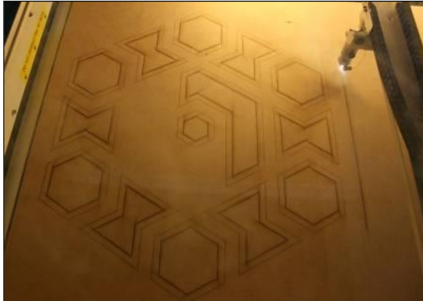
Figure 9.47: Laser cutting the Hexagonal design in MDF design.
