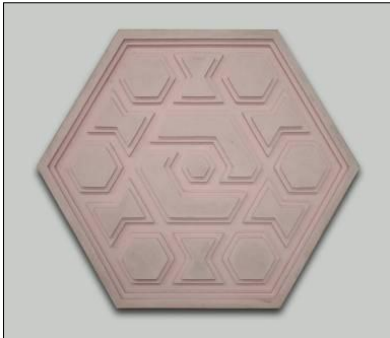
Figure 9.51: Completed Silicone Rubber mould.
