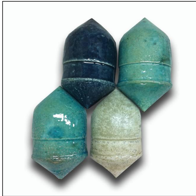
Figure 9.120 Initial glaze tests – Earthenware & Stoneware.
