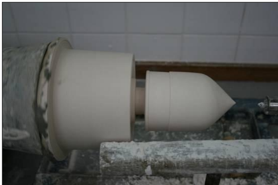
Figure 9.116: Final shaping of plaster model before removing from lathe.
