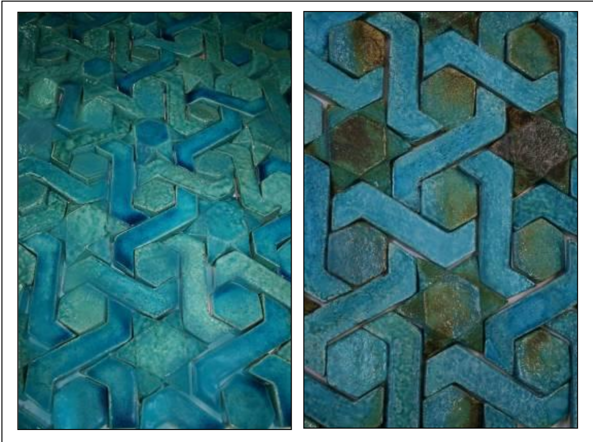
Figure 9.25: Images of glazed and fired tiles, showing variation in tone and colour, due to variation in glaze slop thickness.
