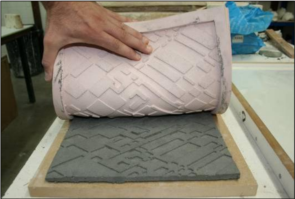
Figure 9.86: Mould being released from concrete cast.
