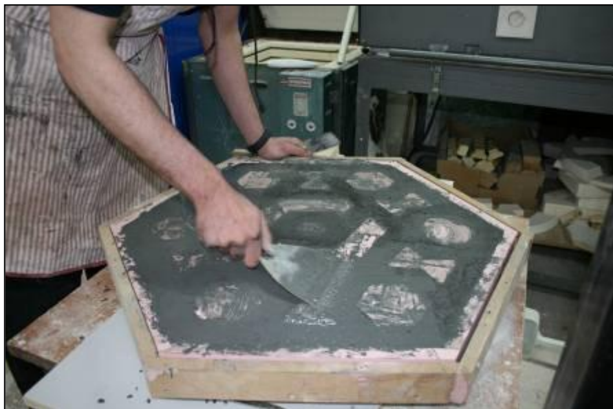
Figure 9.53: Casting Refractory Concrete front face down.
