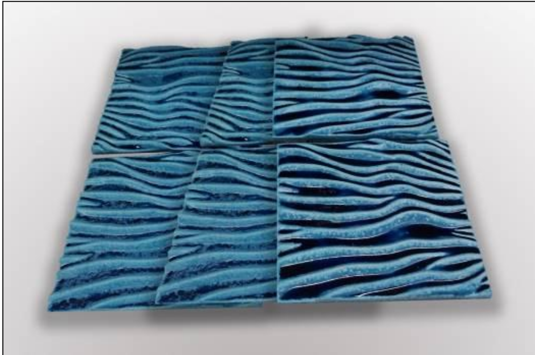
Figure 9.35: Examples of glazed tiles after firing to 1280°C. Note the tonal variation of colour caused by the fluidity of the glaze.
