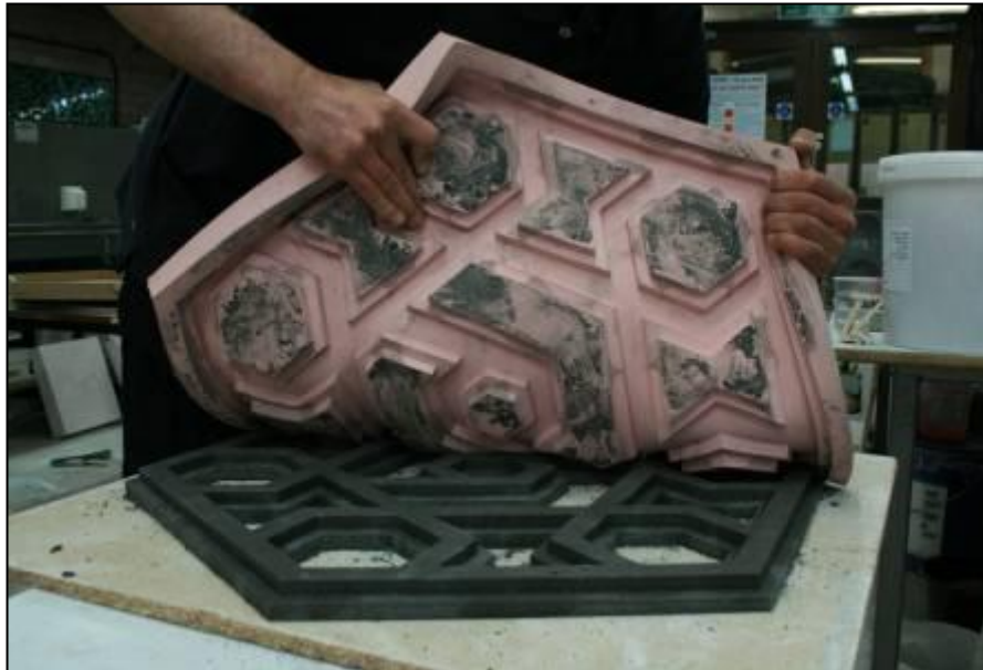
Figure 9.54: Releasing concrete cast from rubber mould.
