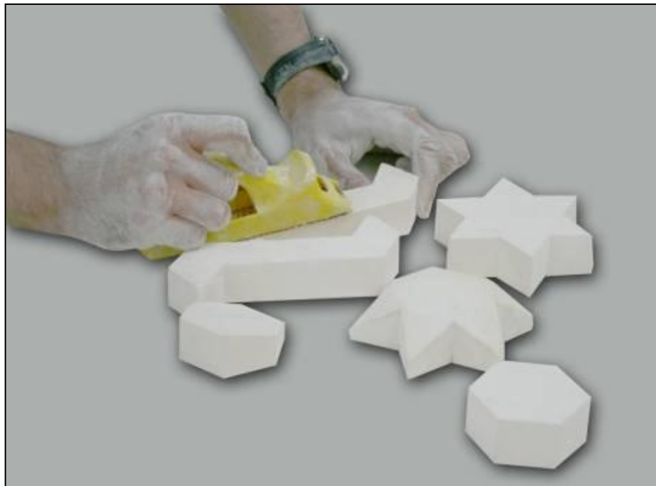
Figure 9.23: Cutting and shaping the surface of 3D plaster models.
