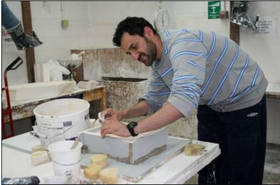
Figure 9.22: Casting a plaster block, from which the 3D tiles will be cut.
