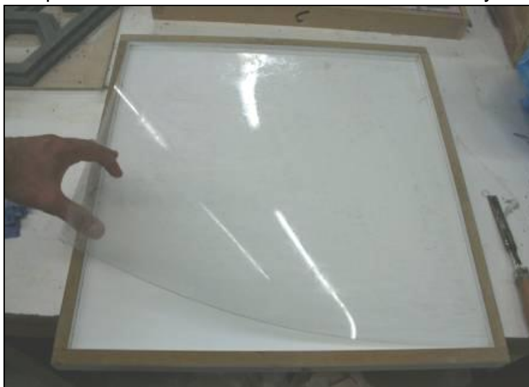
Figure 9.93: Tile casting mould with acrylic sheet base.
