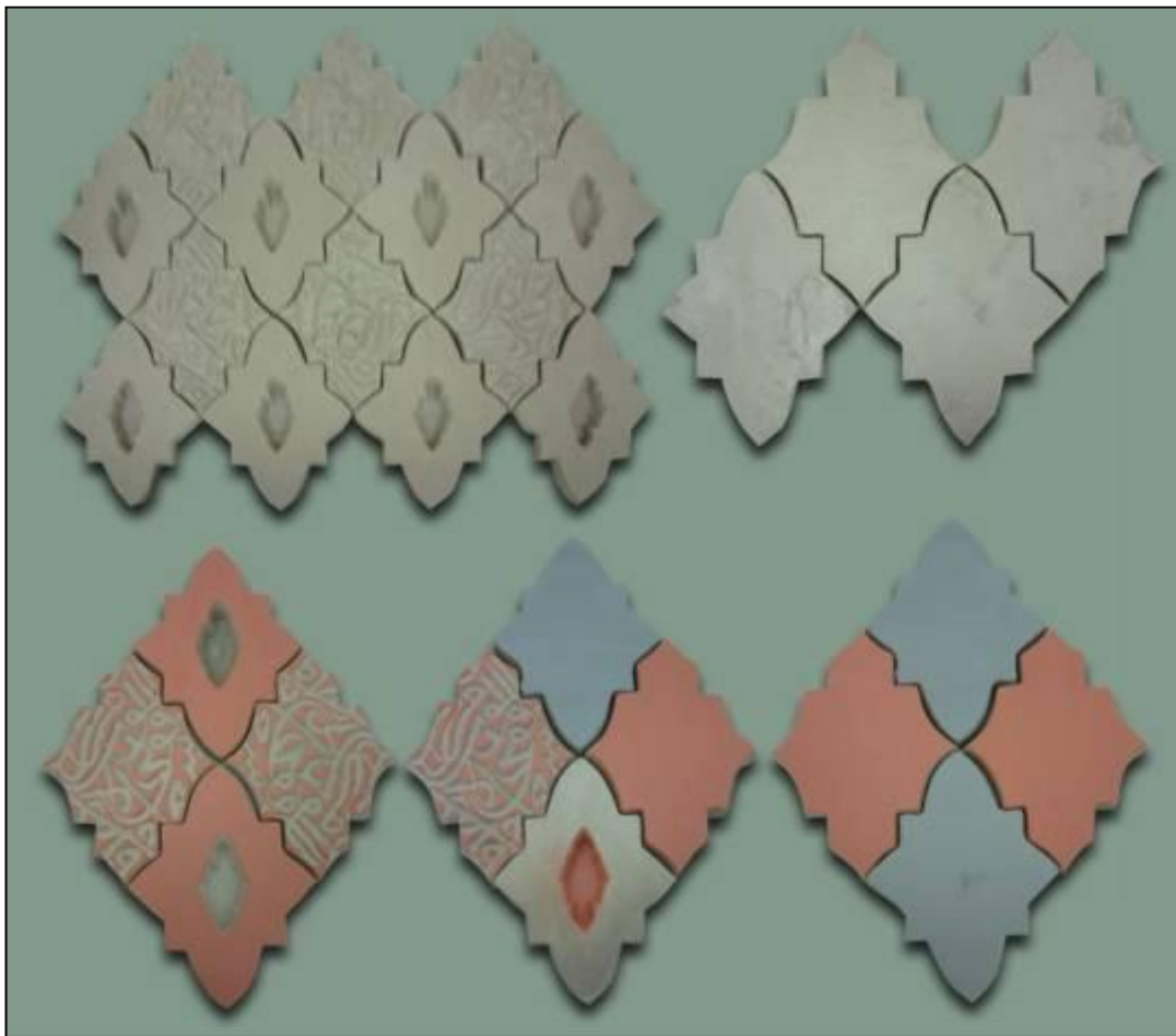
Figure 9.5: Pressings of the tile design and testing the coloured slips.
