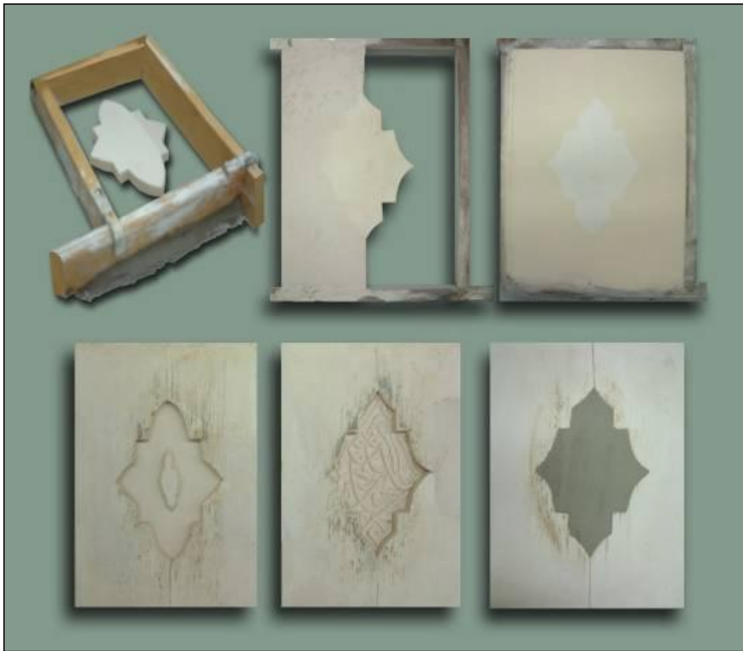
Figure 9.4: Mould making process and pressing the clay into the mould to get the test design.
