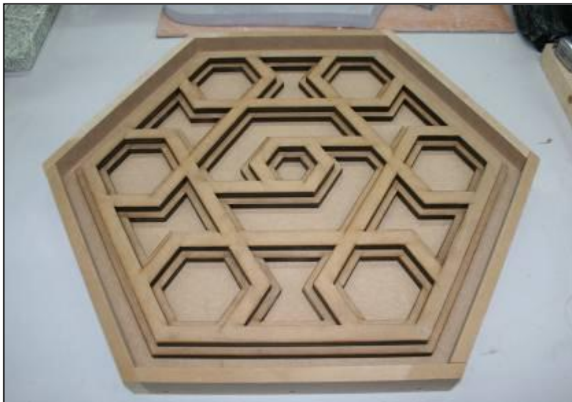
Figure 9.49: Completed MDF model sitting in wooden box, ready for casting in silicone rubber.
