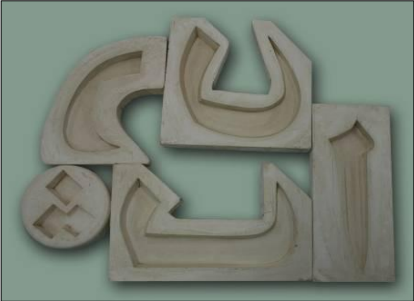
Figure 9.69: Completed plaster moulds of each calligraphy letter-form.
