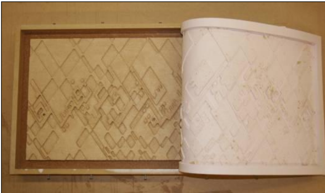
Figure 9.84: Silicon rubber mould being peeled off MDF model.
