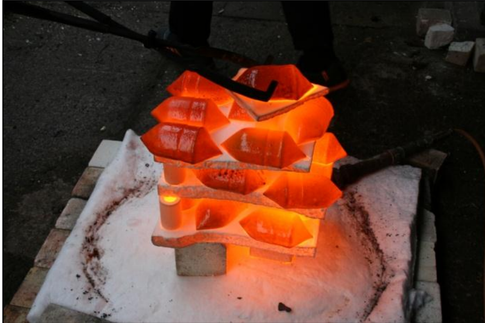
Figure 9.122 Removing Muqarnas forms from Raku Kiln, for placing in sawdust.
