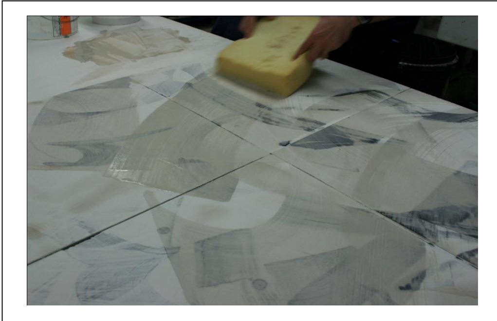
Figure 9.101 Applying thin wash of transparent Earthenware glaze with large sponge.
