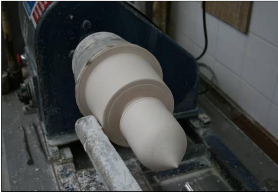
Figure 9.115: 3D dome shaped Muqarnas model being turned on plaster.
