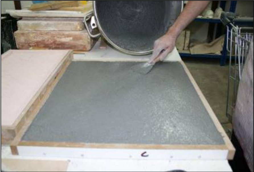
Figure 9.95: Smoothing out reverse side of mould prior to setting.
