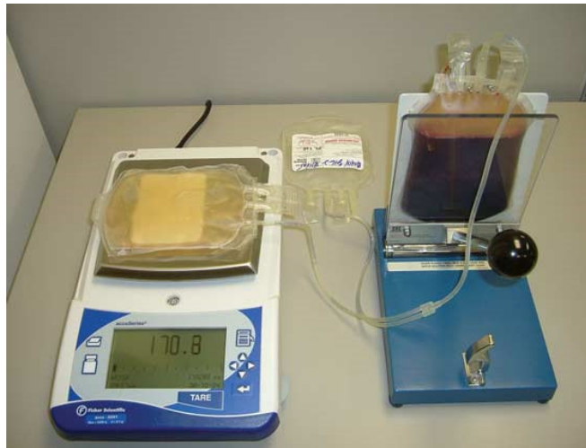
Figura 15. Extrayendo plasma de sangre entera (Acculab and Baxter Healthcare Corporation) (Feldman and Sink, 2008).
