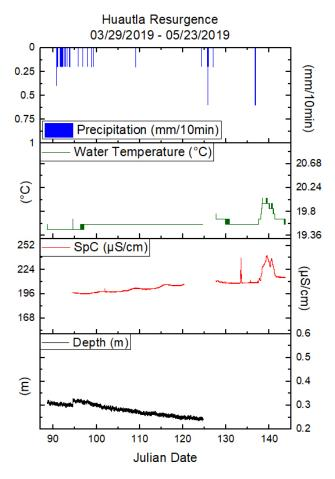
Fig. 5.6 Sistema Huautla Resurgence geochemistry data and water level obtained using HOBO loggers (water level data collection ended prematurely on JD 125 due to equipment access issues) (Source: Created by Author).
