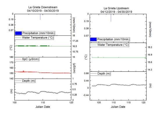
Fig. 5.10 La Grieta geochemistry data and water level obtain with HOBO loggers; left- Downstream, right- Upstream (Source: Created by Author).
