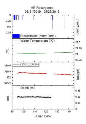
Fig. 5.7 HR Resurgence geochemistry data and water level obtain with HOBO loggers (Source: Created by Author).
