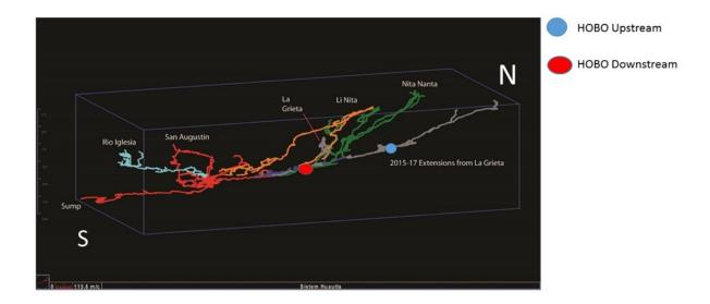
Fig. 4.6. HOBO UL20 Temperature/Pressure Placement in La Grieta, Profile View. (Modified map from Kambesis using COMPASS).
