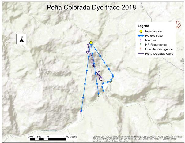
Fig. 5.1 Hydrological pathways observed during the dye tracing of Cueva de la Peña Colorada (Source: Created by Author).
