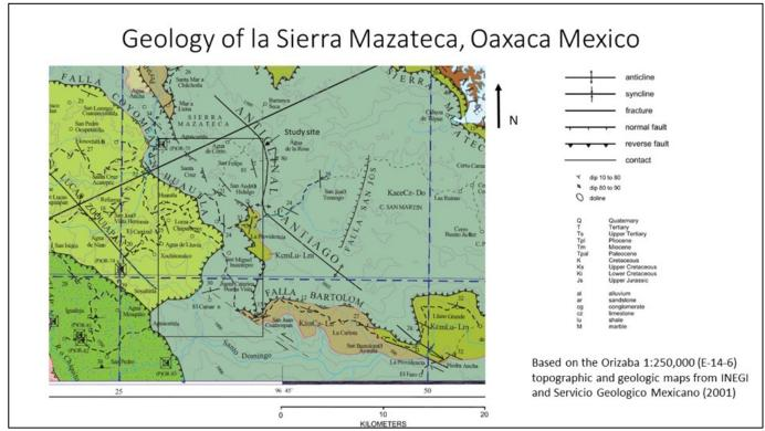
Fig. 3.2. Geology of the Sierra Mazateca, Oaxaca Mexico (Source: SGM 2001).
