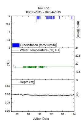
Fig. 5.8 HR Rio Frio geochemistry data and water level obtain with HOBO loggers (only five days of data available) (Source: Created by Author).
