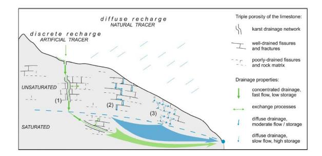
Fig. 2.1. Conceptual model of drainage in alpine karst systems in the Wetterstein Mountains, Germany (Source: Lauber and Goldscheider 2014).
