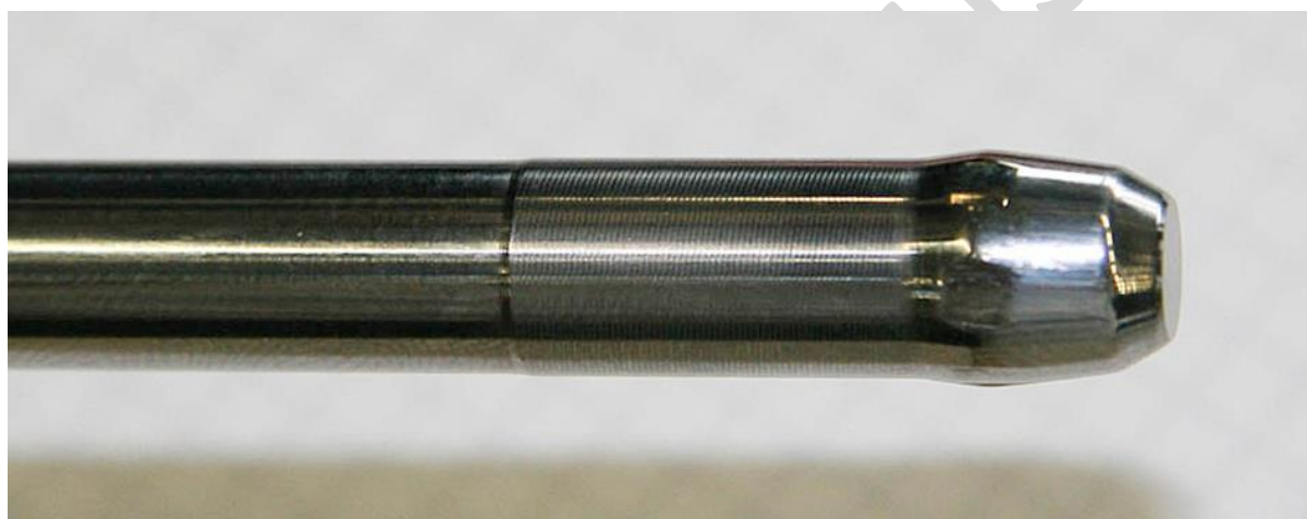
Figure 3. An elliptical button with the negative imprint of lands and grooves.
