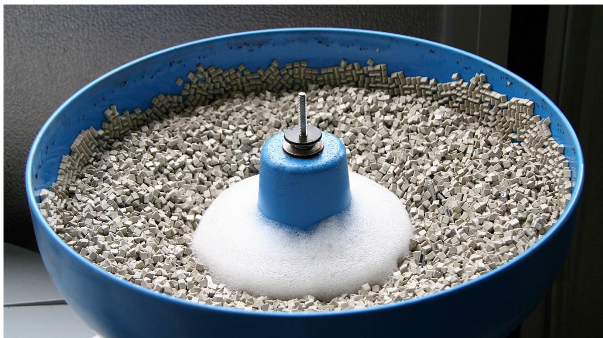
Figure 6. Tumbling process: small abrasive stones and detergent.
