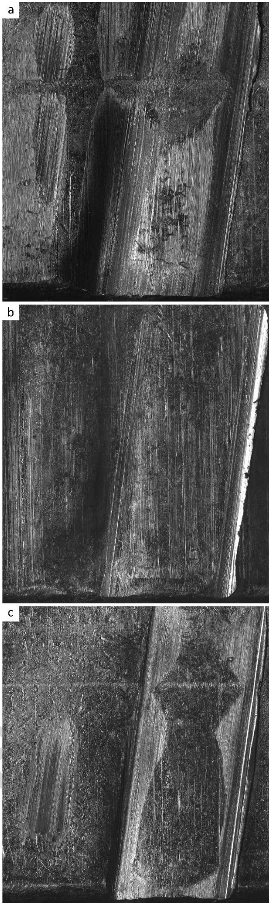
Figure 2. Lands and grooves impressions on the bullets scanned with the Evofinder® ballistics identification system (ScannBI Technology Ltd, version 6.5.0.122) left on the same ammunition (9 x 19 mm Parabellum, Magtech, model 9B, FMJ, 124 gr) by three semi-automatic pistols manufactured by different rifling process: (a) Beretta 92FS (broaching), (b) Walther P99 (button rifling) and (c) Steyr M9-A1 (cold hammer forging).
