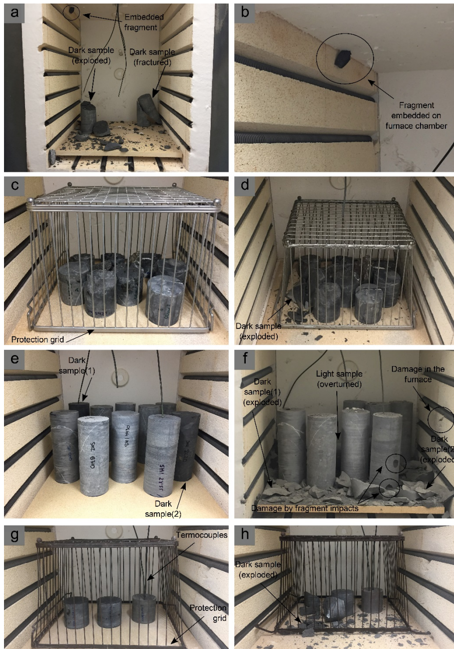
Figure 6. (a) Dark samples exploded or fractured when heated at 400° C. (b) Detail of the fragment embedded in the furnace chamber due to the violence of the event shown in (a). Dark samples before (c) and after (d) heating at 400°C. Note the protection grid used to preserve the furnace. Dark and light grey cores before (e) and after (f) heating at 500° C. Note that only dark cores exploded, and their fragments overturned and damaged the surrounding light grey samples and the furnace chamber. A new set of dark samples before (g) and after (h) heating at 500° C using the protection grid.
