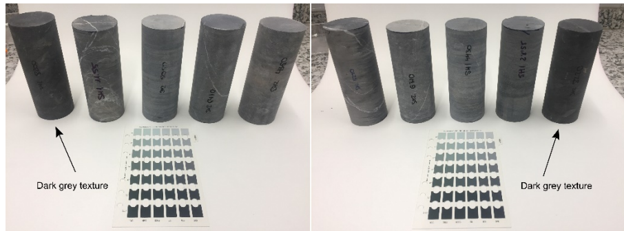
Figure 1. Cylindrical cores from 'Prada' limestones before thermal treatment. Samples with a dark grey texture are identified in the figure.
