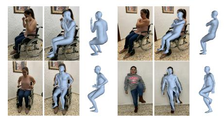
Fig. 4: . The 3D human pose estimation system is able to accurately estimate the human pose even in difficult cases such as persons in wheelchair or scenarios with high self-occlusion level caused by the exercises.
