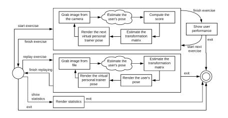
Fig. 1: Flowchart of EVA system. Note that the cloud-based parts are shown in a cloud shape.
