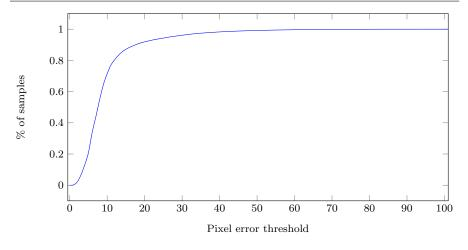
Fig. 13: The accumulated percentage of samples per error (px on a  $224 \times 224$  image) threshold between the 2D points provided by KARD and those estimated by our Human 3D Pose Estimation approach.
