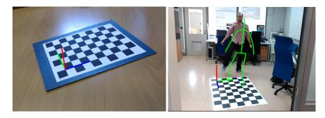
Fig. 2: A chessboard pattern is used as "the trainer's mat". It is a well-known pattern that allows the system to estimate a common 3D coordinate frame. The leftmost image depicts the pattern with the 3D axis superimposed. The rightmost image depicts the personal trainer (skeleton in green) in augmented reality in front of the patient who is imitating them. The personal trainer is rendered *in situ* thanks to the pattern's detection.
