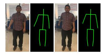
Fig. 3: The 2D poses cannot be used for a robust pose comparison between the user and the trainer because it may eventually fall into a singularity or ambiguous poses such as the depicted in this figure. According to the 2D pose, it is impossible to state whether the patient is rising his arm forward or backward.
