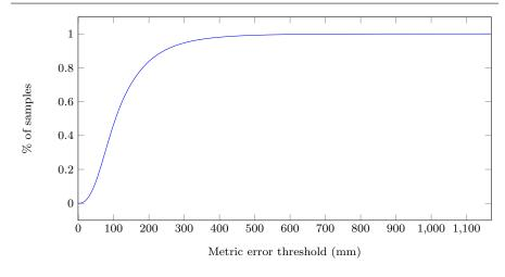
Fig. 14: The accumulated percentage of samples per error (mm) threshold between the 3D points provided by KARD and those estimated by our Human 3D Pose Estimation approach.
