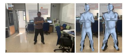
Fig. 6: Performance of the Human Mesh Recovery network feeding it the whole image (center) and the person area of interest detected by YOLOv3 (right-most).
