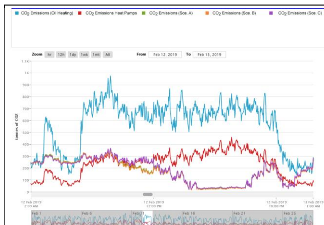
Figure 8. CO 2 Emissions of Oil heating vs Heat pumps in normal operation vs Heat pumps in the three Scenarios
