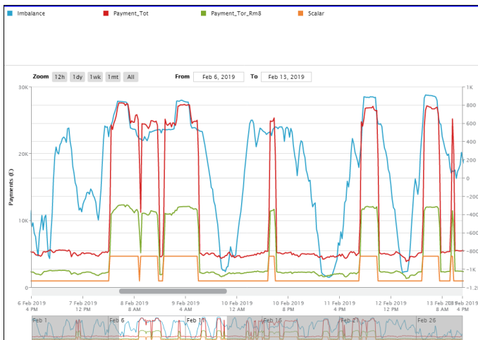
Figure 4. Sum of DS3 Payments (£) in each 30 minutes period and System Imbalance for February 2019
