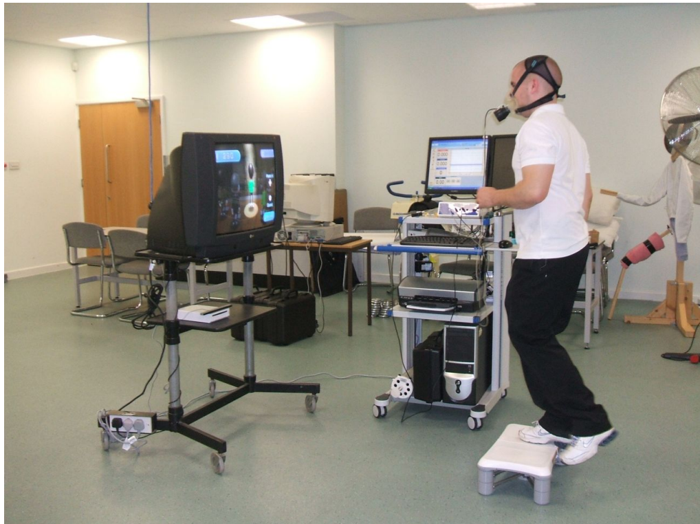
Figure 1. Participant playing Nintendo Wii Fit with raised Wii Balance board. MetaLyzer® 3B in operation.
