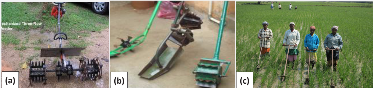
Figure 5.5: A mechanical (motorized) weeder (a) and common types of push weeders (b) being utilized by farmers in the field (c). Photo credit: Sophia Kashenge/TARI-Dakawa.
