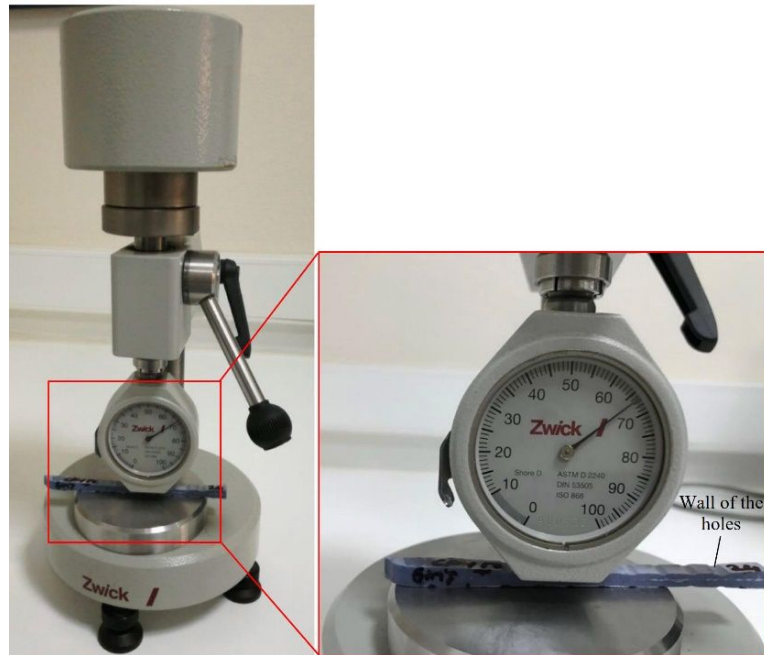
Figure 4: Hole surface hardness measurement
