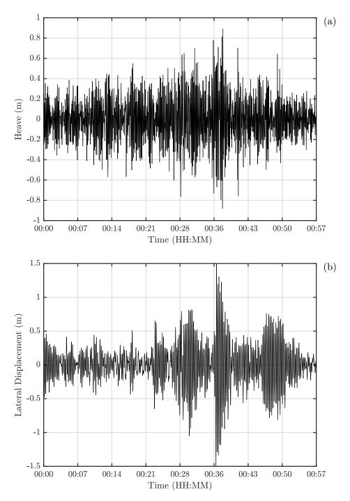
**Figure 8:** Dynamic component of the bridge response between 00:00 UTC and 01:00 UTC on 9<sup>th</sup> January 2015 (a) heave (b) lateral displacement.
