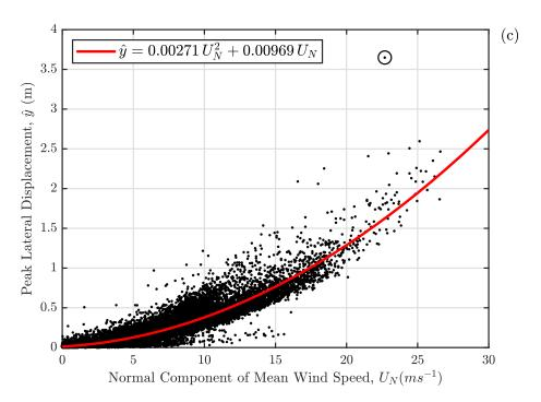
**Figure 4:** Variation of lateral displacement at midspan with normal component of mean wind speed for the year 2015, (a) 10 minute mean (b) 10 minute RMS and (c) 10 minute maximum. A second order trend line is included to indicate the expected quadratic relationship with wind speed. Note the anomalous response is circled in each chart.
