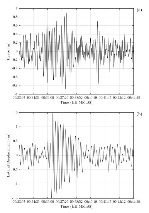
**Figure 9:** Dynamic component of the bridge response showing response to significant gust event (a) heave (b) lateral displacement.
