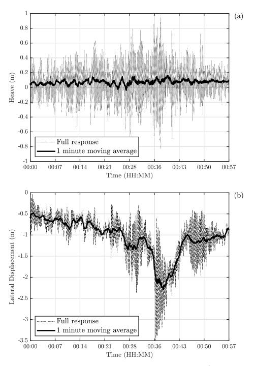
**Figure 7:** Bridge response between 00:00 UTC and 01:00 UTC on 9<sup>th</sup> January 2015 (a) heave (b) lateral displacement.
