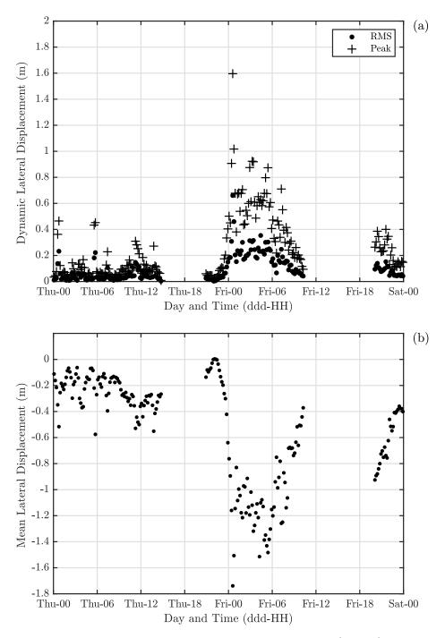
**Figure 5:** Variation of lateral displacement during January 8<sup>th</sup> and 9<sup>th</sup> 2015, (a) RMS and peak response found from ten minute window by removing the one minute moving average (b) mean response found from a ten minute window.
