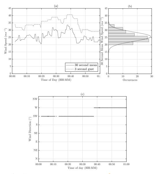
**Figure 11:** Wind data between 00:00 UTC and 01:00 UTC on 9<sup>th</sup> January 2015 (a) wind speed showing 30 second mean and corresponding 3 second gust (b) distribution of 30 second mean wind speed and normal distribution for comparison (c) 30 second mean wind direction.
