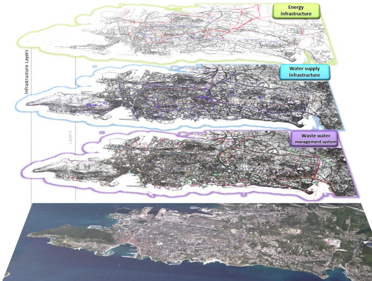
Figure 12 - Superimposed Energy, Water, and Waste Water Infrastructure Context of the Micro grid
