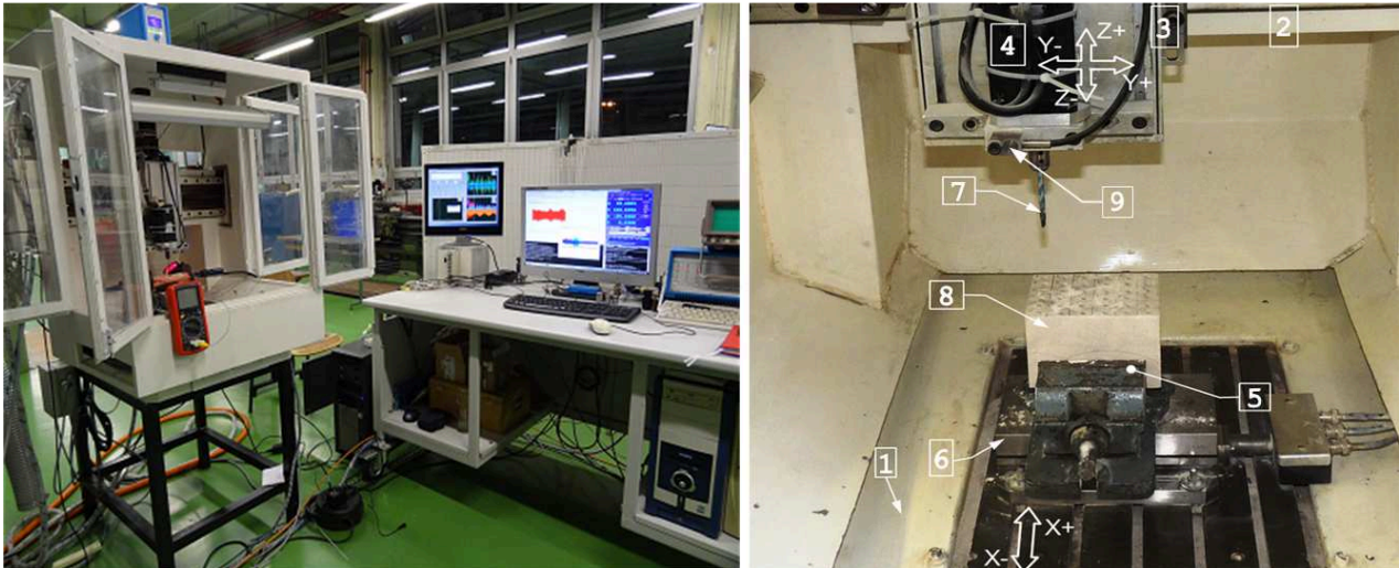
Fig. 1. Experimental setup - work area and sensor placement. (1) X axis feed drive; (2) Y axis feed drive; (3) Z axis feed drive; (4) main spindle drive; (5) workpiece fixture; (6) three axis force sensor; (7) test drill; (8) stone workpiece; (9) AE sensor
