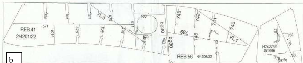
Slika 7. Rezanje limova u brodogradilištu (a) i dio od kojeg su uzimani uzorci (b) Fig. 7 Plate cutting in shipyard (a) and the plate from which the specimens were extracted (b)
