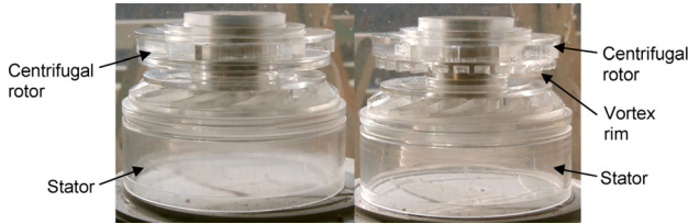
Fig. 3 Centrifugal and centrifugal vortex pump stage made of Plexiglas for experimental research
