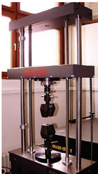
Fig. 4. Screw-drive testing machine Messphysik BETA 50-5.
