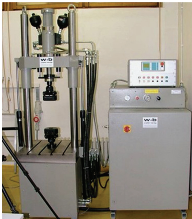
Fig. 5. Servo-hydraulic testing machine LFV-50-HH.
