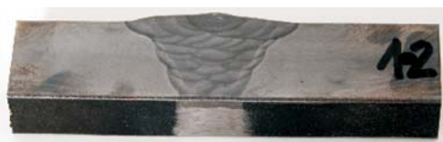
Figure 5 Macro cross section of RD-test (specimen 1-2) Slika 5. Makropresjek RD - probe (eproveta 1-2)
