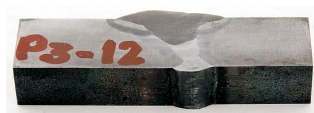
Figure 10 Macro cross section of specimen P3-12 Slika 10. Makropresjek epruveta P3-12
