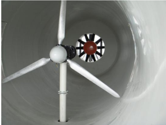
Fig. 8: Wind turbine in the chamber.
