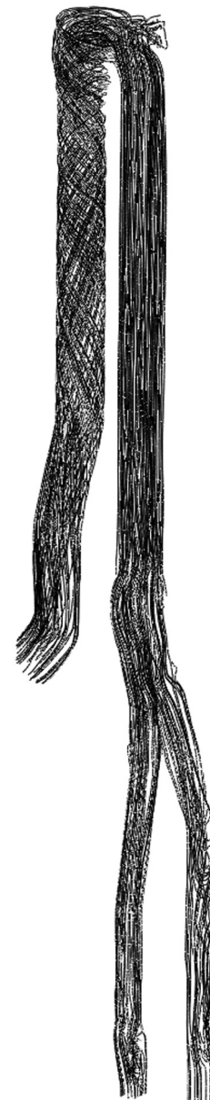
Fig. 2. Flow streamlines inside the calculated calciner.
