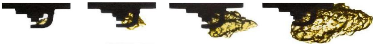
Figure 13. Visualization of the early flame kernel growth from the experiment [55] indicating the effects of local bulk flow and turbulence in the vicinity of the spark plug.
