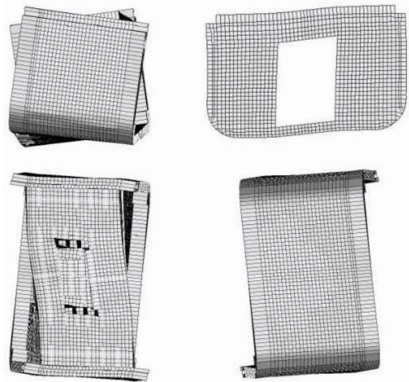
Figure 21 Lateral, axial, bird's-eye and fish views on deformed engine room superelement Slika 21 Bočni, uzdužni, ptičji i riblji pogled na deformirani superelement strojarne
