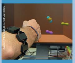
Transfer learning technologies developed at Bielefeld University enable a rapid recalibration of cuff electrodes for hand prosthesis
