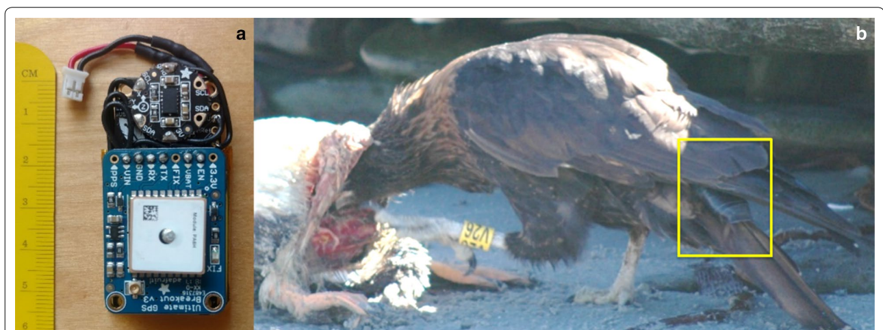
Fig. 5 The TWLogger inertial movement datalogger with GPS prior to encapsulating in heat shrink for deployment (Fig. 5a), and a banded caracara wearing a tail-mounted TWLogger (Fig. 5b) while feeding on a gentoo penguin carcass at the seabird colonies site
