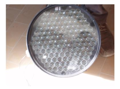
**Figure 3.3:** The front plate of the CT1 camera. In front of PMTs are the Winston cones – designed to minimize the dead-space between the photocathodes of the PMTs. Picture by Nikola Godinović from Split.
