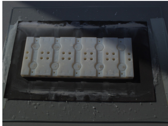
(b) Wet sanding process
