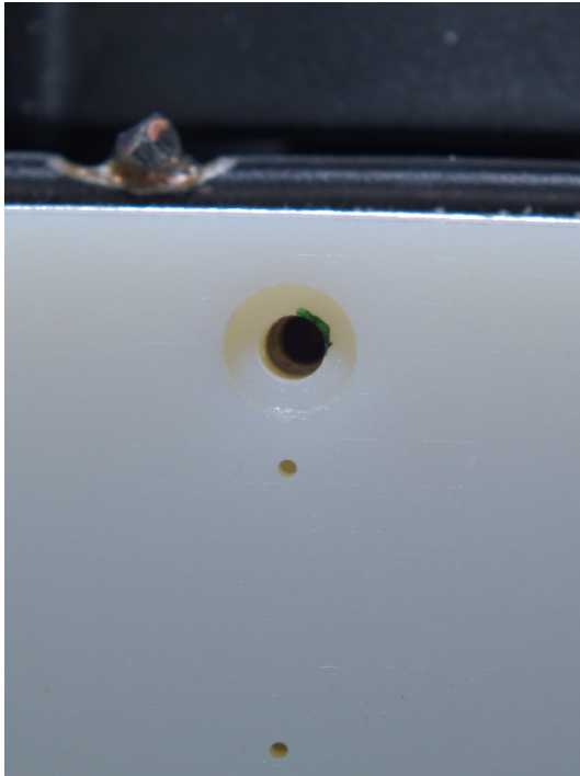
(a) Tolerance error of the threads
