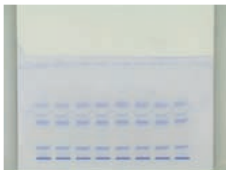
Fig. 3.5-4: shows eight melamine spiked milk samples (each with 1 µL applied), stained with Wuster's blue reagent
