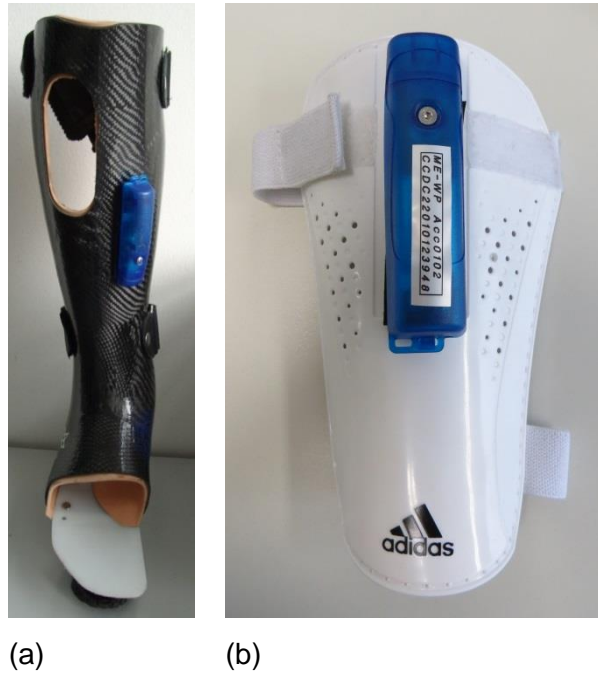
Figure 6-1: Position of accelerometer on HEPHAISTOS orthosis (a) and on shin guard (b)
