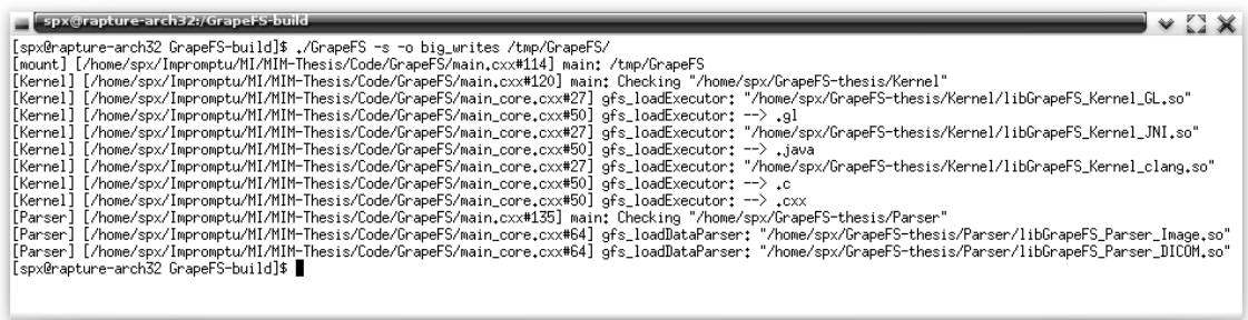
Figure 19: Mounting GrapeFS. Any mount point can be chosen as a startup parameter. The "-s" option is mandatory to prevent multiple FUSE threads. Currently not all components of GrapeFS are thread-safe. The "big_writes" option significantly improves write throughput by reducing the number of write calls to user-space.
