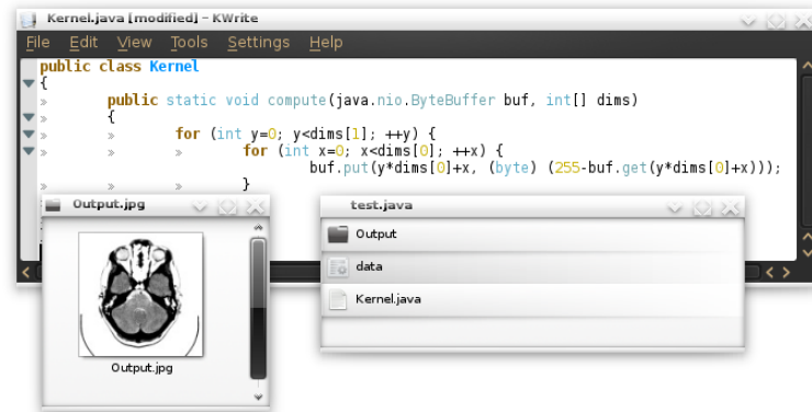
Figure 32: Example for data processing using the GrapeFS Java front-end. The processing folder has been created using the .java extension. Java code is written to the Kernel.java file. Within the Java code the data is handled using a ByteBuffer. As with every other processing front-end the processing result can be accessed using the output folder.
