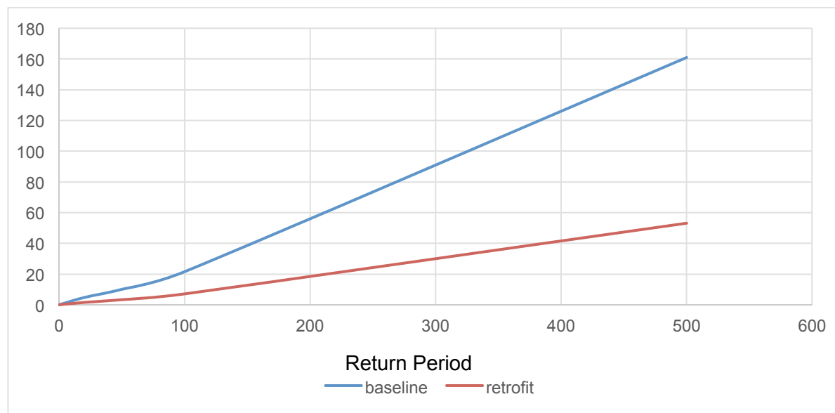
Figure 53: Loss Return Period Curves Pre and Post housing retrofitting Project (in Million USD)
