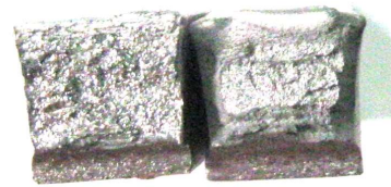
Figure 4 – Macrostructure of a specimen tested for impact toughness after quenching and high tempering
