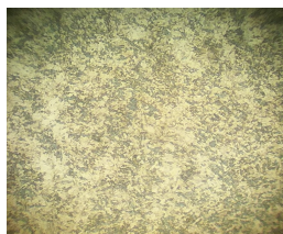
Figure 2 - Microstructure of AISI 420 steel in the vertical direction at 980 °C, \times 200
