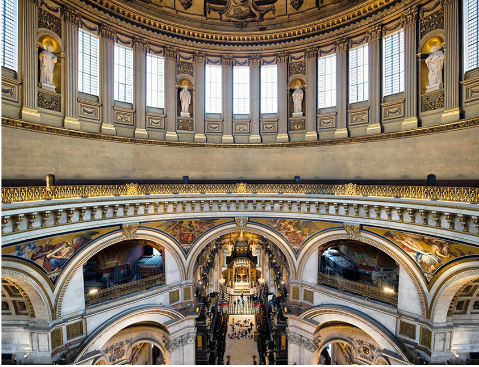
Figure 2.1: Whispering gallery in St. Paul's Cathedral. Acoustic waves at particular frequencies travel along the curved wall and are audible along the entire periphery. The above photograph is taken from [35].
