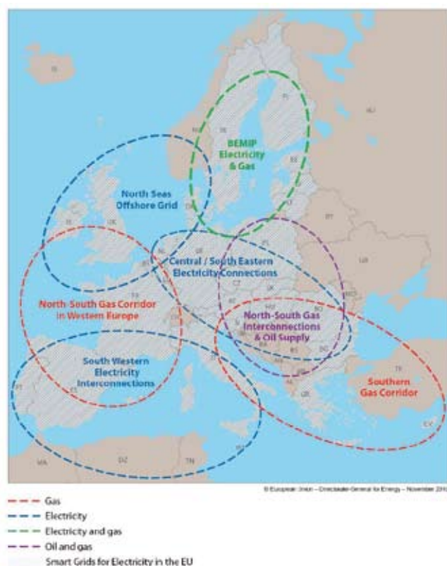
Figure 5: European Commission priority corridors for the improvement of electricity, gas and oil infrastructure
