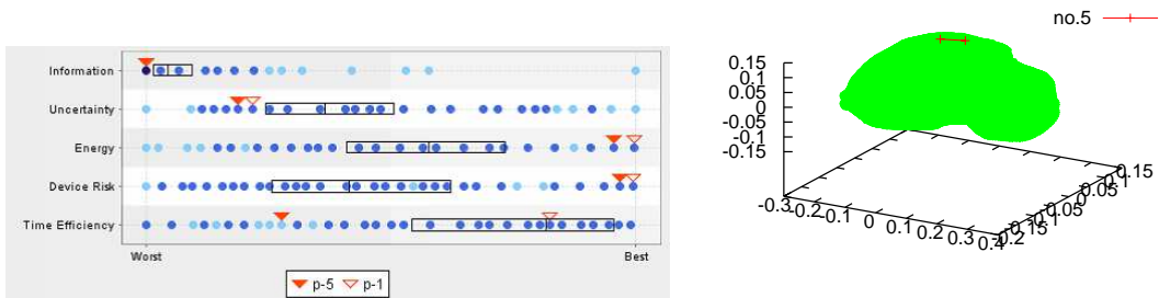
Fig. 13: An example of alternative analysis (left) and the designed path no. 5 (right) : when the user specifies large preference on both obtainable information and device risk.
