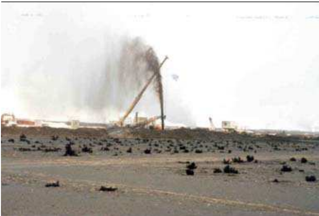
Figure 14. A damaged oil well still gushing oil and gases after the fire has been extinguished.
