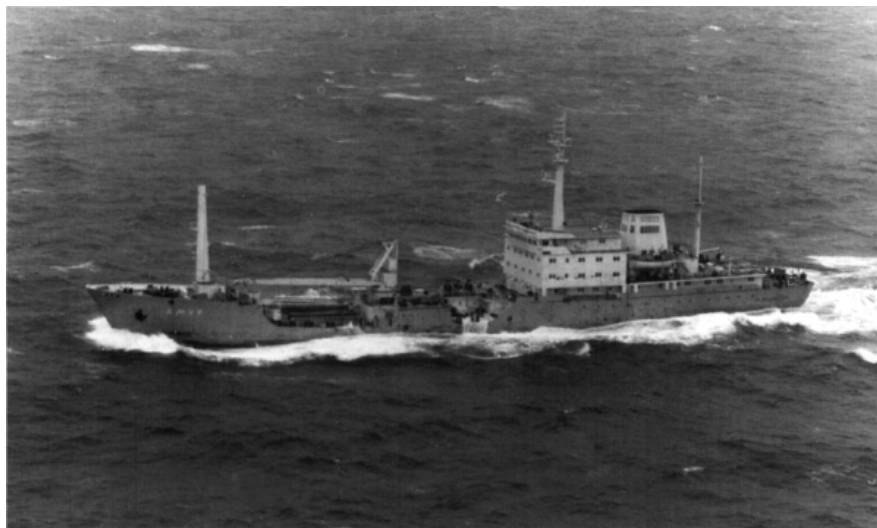
Figure 2-7: The Project 11510 class technological tanker "Amur", sister ship to the "Pinega" ( Bellona, 1996 )
