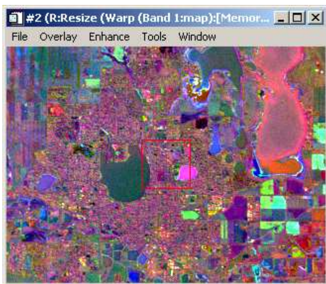
Figure 4: Abundance of endmembers from AVIRIS image. Red is urban, green is irrigated agriculture and blue is water.
