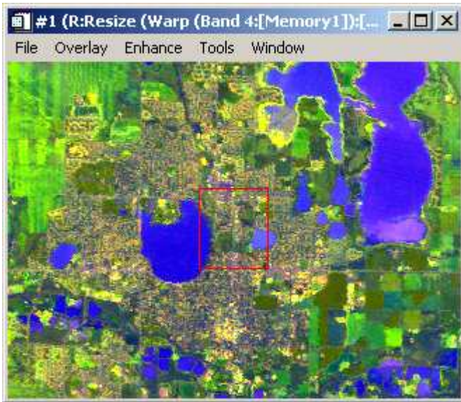
Figure 5: Abundance of endmembers from TM image. Red is urban, green is irrigated agriculture and blue is water.
