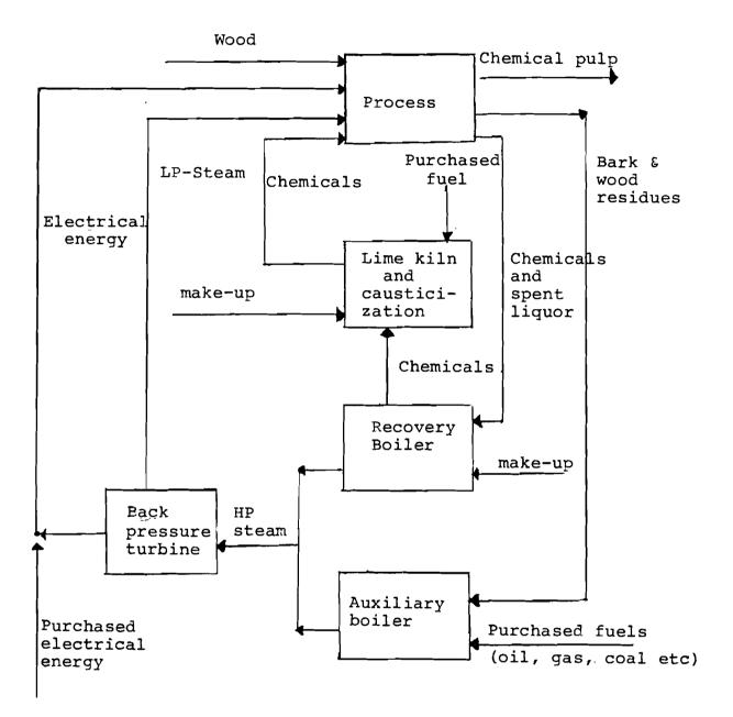
Figure 3. A simplified flow sheet of energy and chemicals in a kraft pulp mill.
