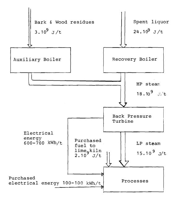
Figure 4. Overall energy balance in a kraft pulp mill. (Per ton of air dry pulp)
