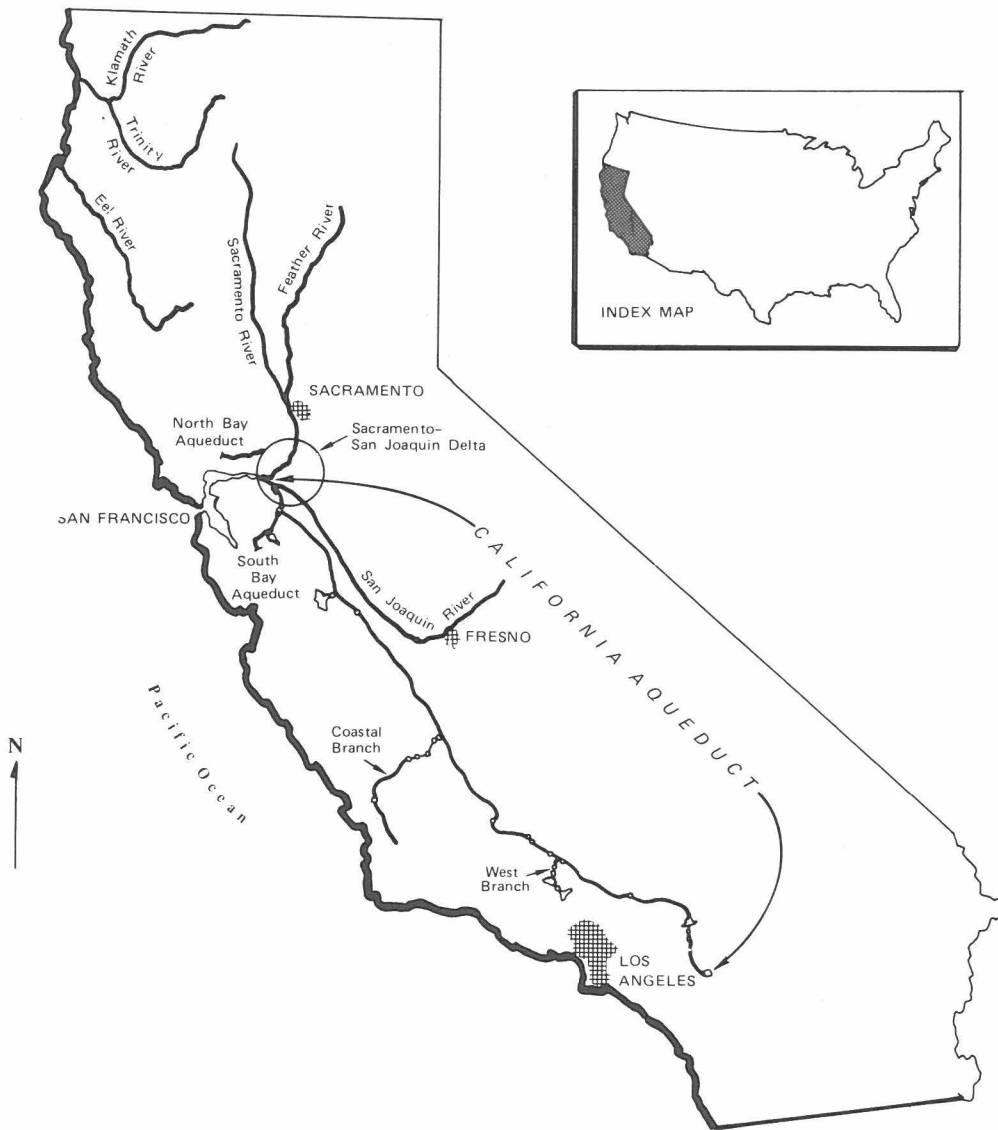
Fig. 1. The California State Water Project.
