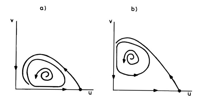
Figure 3: Two types of limit cycles
