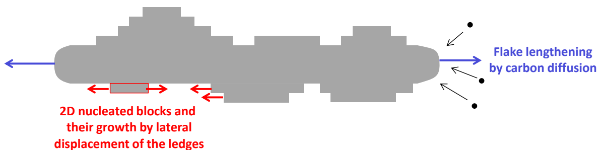
Fig. VI-5. Schematic of the growth and thickening processes of a graphite flake (adapted from [AMI13]). Lengthening of the plate is controlled by carbon diffusion to the tips. Thickening proceeds by 2D nucleation of new growth blocks onto the basal faces of the plate and their lateral growth parallel to the basal faces..
