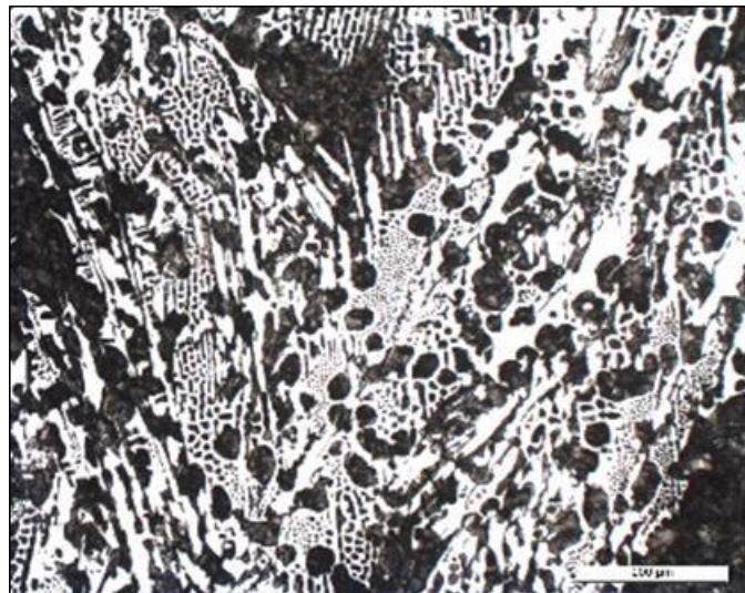
Figure IV-5. Optical micrograph: appearance of cementite (white) on the metallographic etched section of a mottled CGI.
