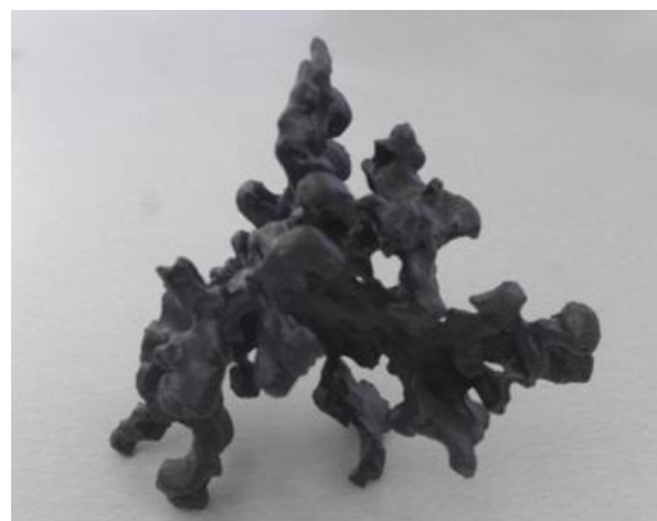
Figure IV-17. Photograph of a 3D printing of graphite in a compacted graphite eutectic cell. The model was built from a tomographic study [CHU15].
