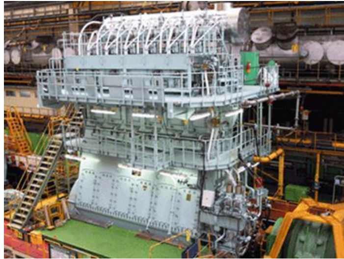
Figure I-2: The biggest or nearly so (Wärtsilä X62 engine)
