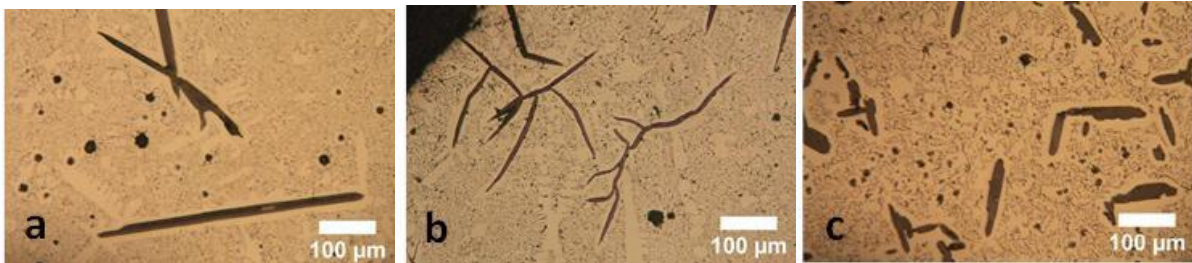
Figure VII-7. Primary graphite precipitates in Fe-C alloys similarly processed under air with no addition (a), Sb (b) and Ce (c) addition [THE13].
