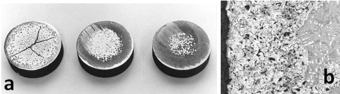
Figure III-8. (a) metallographic section of a cylinder 38 mm in diameter quenched at various times during solidification of a LGI. (b) micrograph of the outer fully solidified shell (Courtesy F. Mampaey).
