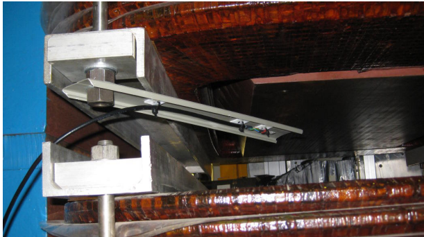
Figure 2: POMPOM #2 installed in D2. The sensor PCB itself is the white chip to the right of the final cable-tie.
